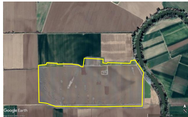
Fig. 3. A detailed UAV composite orthophoto (yellow border) overprinted onto a satellite image, clearly shows that the distribution of individual liquefaction features (gray spots) coincides with an abandoned and filled bend of Pinios river. The current riverbed is visible at the right part of the map.
