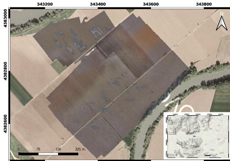
Figure 2. An example of orthorectified image of the liquefied areas (gray spots). Images from a series of high flying UAV campaigns have been combined with orthophotos from the Cadastral project of Greece.
