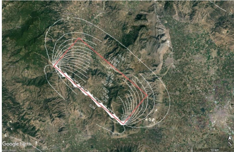
Fig. 7. A preliminary model of the seismic source is showing vertical displacement on the ground. Surface fault trace projection between the villages Zarko and Megalo Eleftherochorion.
