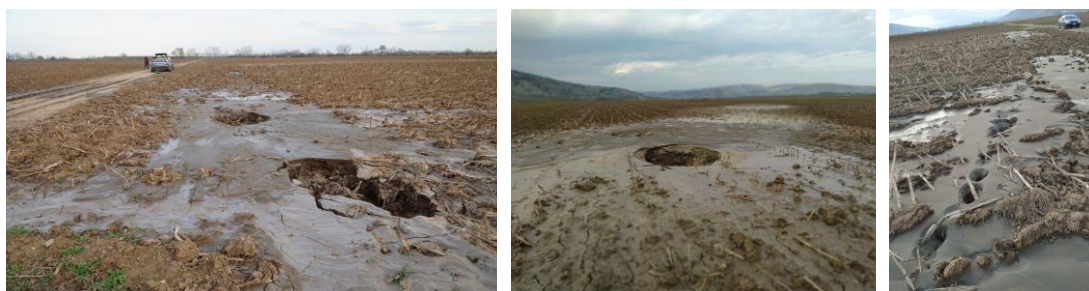
Fig. 1. Eexamples of sand flow and craters in the liquefied area SE of Pineiada village.
