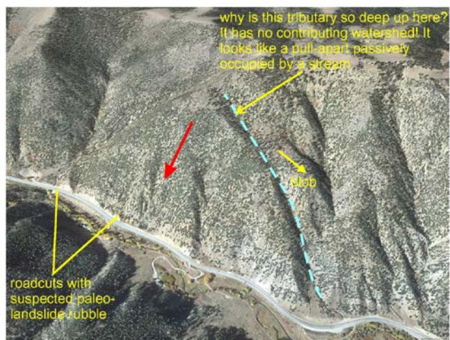
Fig. 0-2. Google Earth oblique image of the west valley wall of Poncha Creek, at the site of the roadcuts exposing low-angle shear zones and pervasive fracturing (lower left). The distinct shear planes at the base of the roadcut dip out of the slope at a relatively shallow angle, raising the possibility they are landslide shear planes, not tectonic faults. The entire rock mass here is shattered over a broad area, which does not show the core vs damage zone pattern typical of tectonic faults. Instead, the rock mass appears to have been shattered by a uniformly-applied external force. The ridge above the roadcuts has some anomalous tributaries that cut into the slope at an angle oblique to the fall line, which appear to be structurally controlled.
