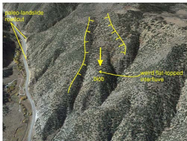
Fig. 0-3. The slope above the landslide contains anomalous sidehill gullies and scarps (yellow) that are more parallel than perpendicular to contours. One interpretation of these odd gullies and the flat blob between them, is that they represent a downdropped gravity block above a slope that has failed outwards downslope. This would be like the headscarp graben or pull-apart zone in a landslide. However, the fact that the graben is still preserved on the steep slope means that the rock mass did not slide very far downslope. This accords with the deformation observed in the roadcut.
