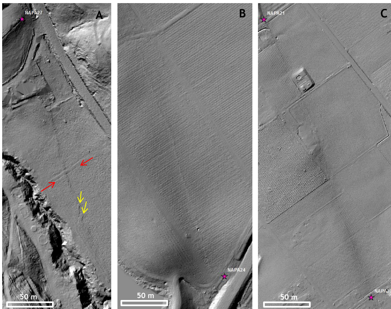
Figure 13: Some outstanding evidences of fault rupture associated with the Napa earthquake as they can be observed on the LIDAR (source: USGS) along the A trace. A: In the northern section, one can observe the left-stepping fractures (yellow arrows) and the dextral offset of the path (red arrow); B: In the middle section, the fault rupture cuts the vine rows where we could measure a 30 cm dextral displacement of a fence (NAPA24 waypoint); C: Along southern section of the rupture, south of Highway 12, the rupture coincides with a gentle scarp facing to the east (underlined by hillshading).
